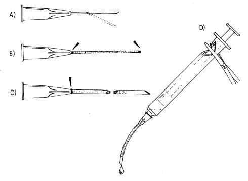
disposable needles which have an aluminium insert, if the filter is to be reused, since electrolyte solutions will cause corrosion and hence contaminate the filter.
